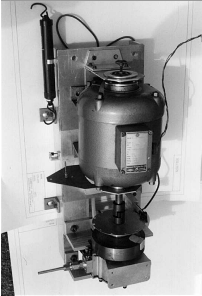
Fig. 10.9 Counterbalancing the mass of the dynamometer by suspending it on its axis eliminates both radial and axial forces on the trunnions and allows the accurate zeroing of the torque datum called for in pumping loss tests
