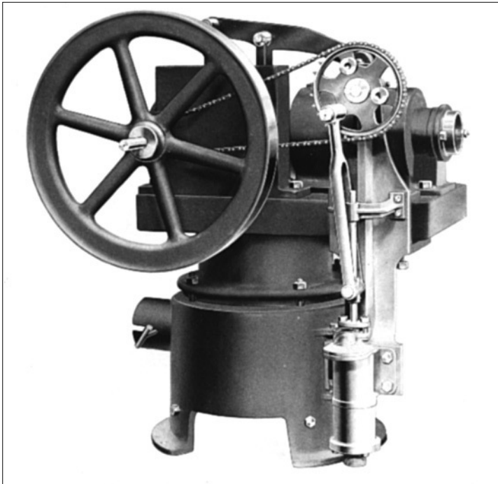
Fig. 2.13 Coal-fired Robinson engine, ca 1908, with attached chain-driven water pump. (Source unknown)
