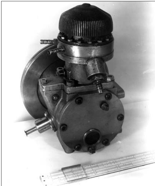
Fig. 4.2 Exterior view of the single-cylinder Philips' 2 h.p. air engine. The gas burner has been removed for clarity. Reproduced with the permission of Philips Electronics BV
